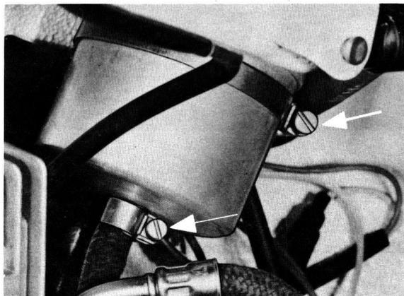
DEPOSE ET REPOSE DE L'ACCUMULATEUR D'ESSENCE
